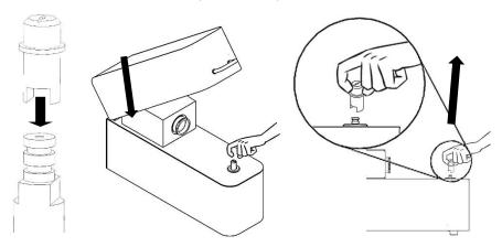
\*\* The two black O-rings, on the main pole that holds the tips, are tend to dry after a while especially because of weather changes. In case the holding tips does not come out smoothly you can apply a little of Vaseline or Lobello lip balm stick on the O-rings.
